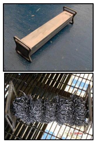
Currently, most drilling rigs use "particle collectors" to support a smooth drilling operation and to prevent damage to the pumps. The available designs in the market use passive magnetic technology to collect as many shavings as possible, employing passive magnetic methodology. The collectors are heavy, requiring cranes to lift and position, while only collecting on the bottom of the ditch. This design misses potentially 36% of metal particles suspended in the mud column near the surface.
