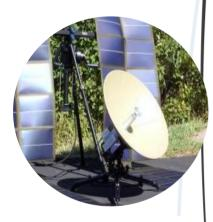
T2 Portable Communications Packages are compact size, light weight, and selfpowered, and support secure voice and data connectivity in the most remote locations around the world. They are self-sustained by off the grid sources -vehicle, solar, wind, and hydrogen fuel cell -- ensuring reliable communication through extended periods in virtually any environment. The T2 system is designed to connect people in even the most rugged environments. Video and radio options are available.
